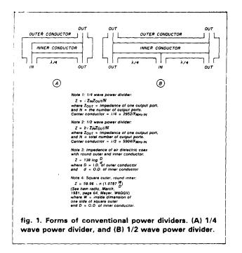
should perform equally as well as the others. At each end of a 1/2 wave four-way power divider, the impedance is one-half the impedance of each output port. This will be 25 ohms for 50 ohm feedline or 37.5 ohms for 75 ohms feedline. We simply extend the matching section, at each end equally, to the desired length, at the impedance of  $Z_{OUT}/2$ . (I will be using this design in my 432 MHz EME array now under construction.)
